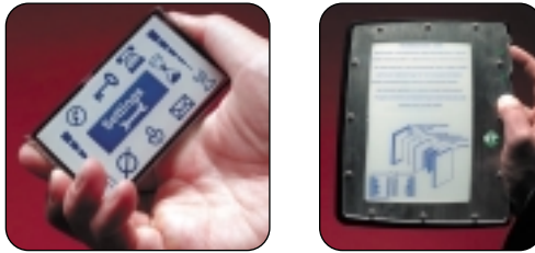
Figure 3.5: Electrochromic displays developed by NTERA with ink-on-paper qualities.
