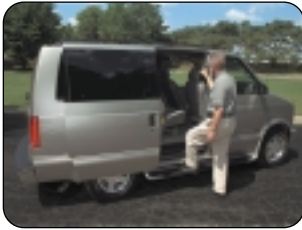
Figure 5.2: The launch of vehicles by GM incorporating a thermoplastic nanocomposite step to assist entry and exit from the vehicle. Step-assist is the first automotive exterior application of this lightweight, high performance and affordable material.
