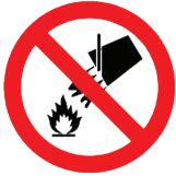
Do not extinguish with water
